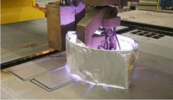
A plasma cutter slices through steel at Quonset. Journal photo by Steve Szydowski
